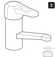
Attach the diverter valve to the faucet using any included adapter rings necessary. Be sure to clean any exposed threads and apply plumbers tape to prevent leaks. If installing to a faucet, please contact your dealer for informationon a specialty adapter that may be required.
