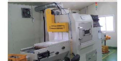
Plates sand blasting Technology
